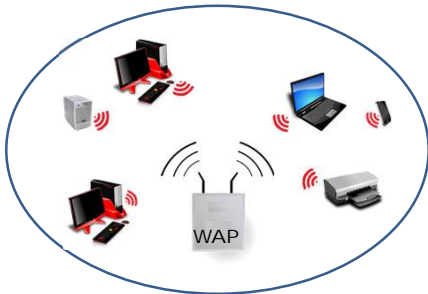
Wireless Access Point (WAP) Creates Wi-Fi connections at the physical layer.
